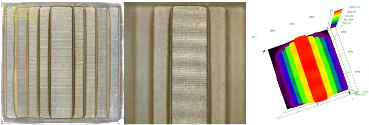
Figure 7.2.16 3D printing from a composition TPO-L + UDMA/TEGDMA 7:3 + AFCT
