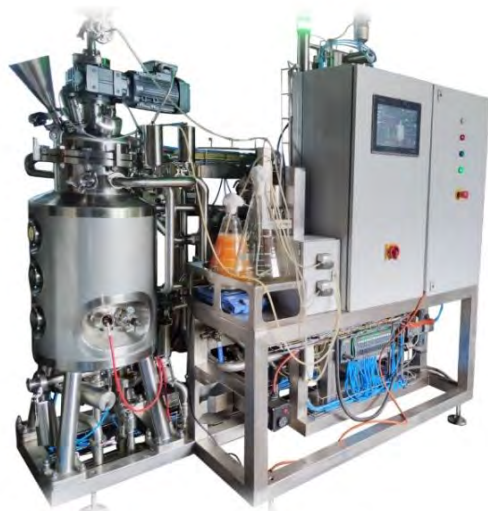
Figure 11.15.1. Bioreactor with continuous nutrient supply for microorganisms and uninterrupted bioprocessing.
