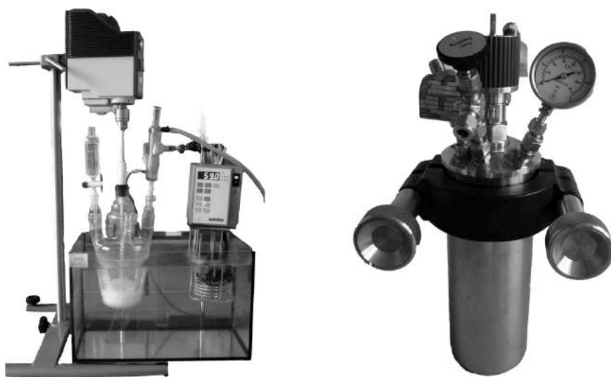
a) b) Fig. 2 The apparatus for the synthesis of the TS-1 catalyst: the glass reactor (a) and the Berghof autoclave (b)
