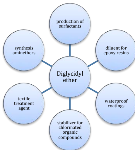
Fig. 15 The application of diglycidyl ether
