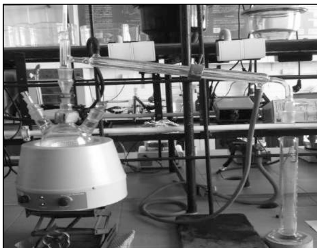
Fig. 1 The simply distillation of limonene from orange peels
