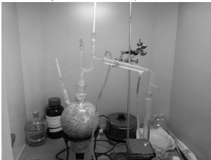
Fig. 8 Scheme of apparatus for steam distillation
