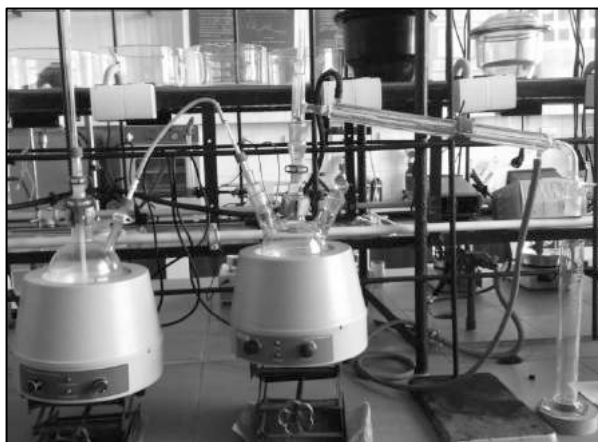
Fig. 2 The water steam distillation limonene in the laboratory scale
